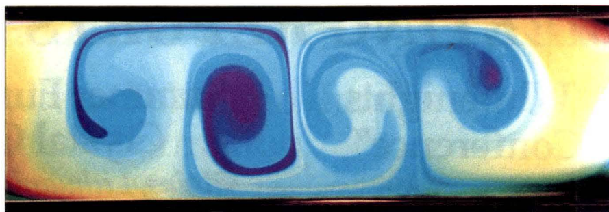
Fig. 2 Convection just above onset in a rectangular film. The colours map the nonuniform film thickness which is advected by the flow. One can make out the steps in colour due to the smectic layering.
