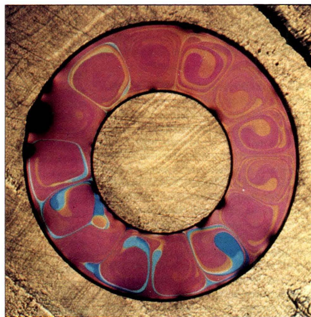
Fig. 3 Convection in a nonuniformly thick film in an annular geometry, with a radial driving force
